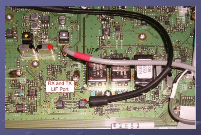
The 10.695MHz LIF port connects to the output of the 2<sup>nd</sup> Mixer and is routed to the back panel and terminated with an SMA connector. Ground is provided by the screw just above the cable.
