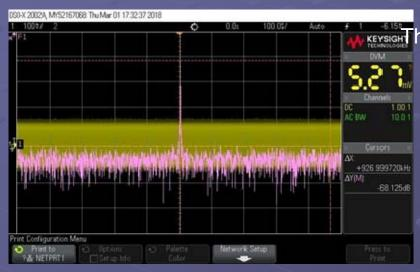
he frequency stability and the phase noise of a crystal cannot be duplicated without some major expenses in DDS and time base circuitry. A lot of the cost-effective and commercially available oscillators have severe phase noise and stability issues. Crystal oscillators allow us to keep the budget low and the quality of the LIF high. The flexibility of the variable IF that DDS allows for, has now been programmed into the software running on the Pi.
