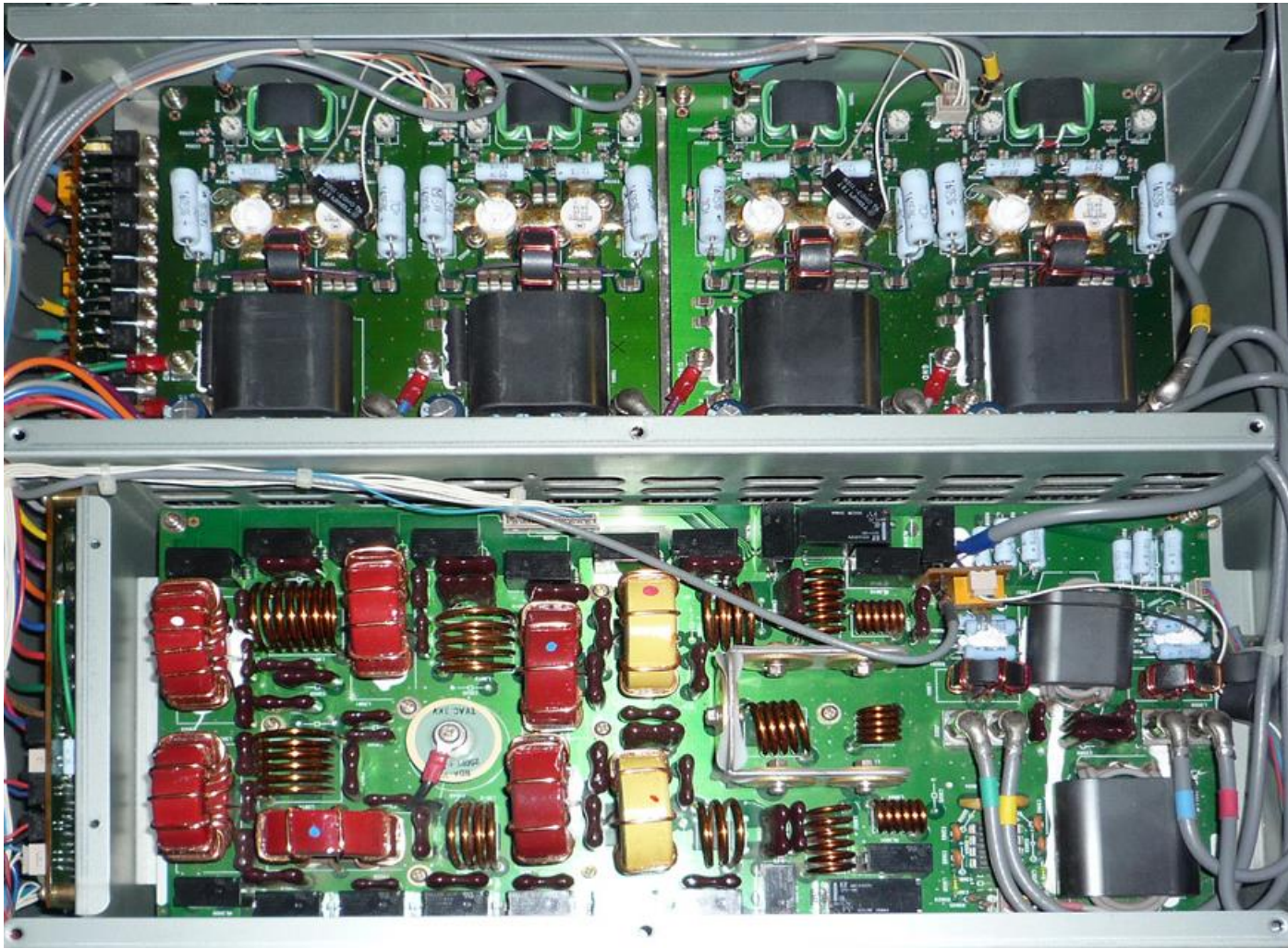
Top: 1kW PA stage (4 X 250W). Bottom: LPFs for all bands 160 - 6m.
