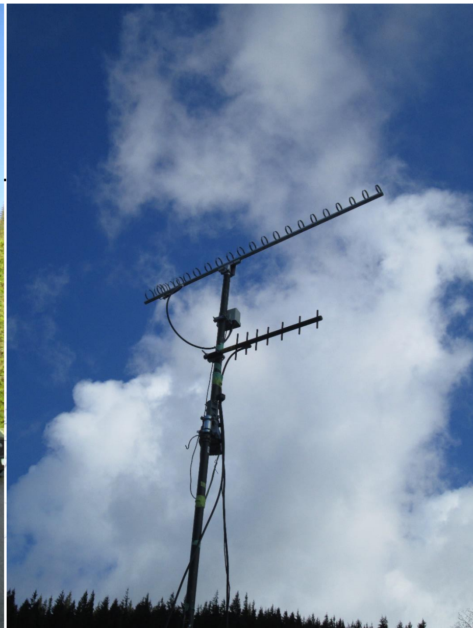
Roving on 927 and 1296 Mhz in CN89ji “Near Max Effort” with rotor, preamp for 1296, medium mast
