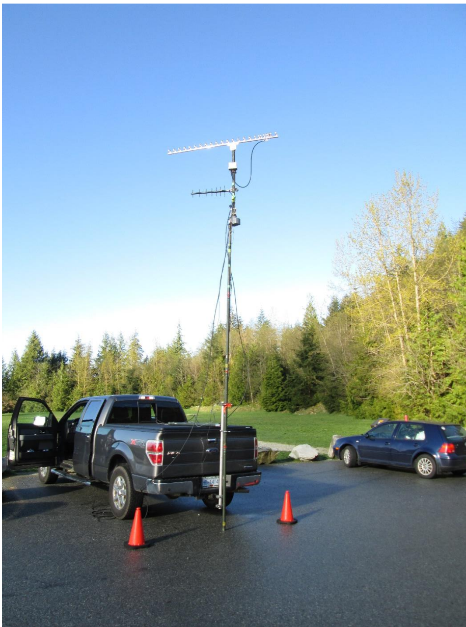
Roving on 927 and 1296 Mhz in CN89ji “Near Max Effort” with rotor, preamp for 1296, medium mast
